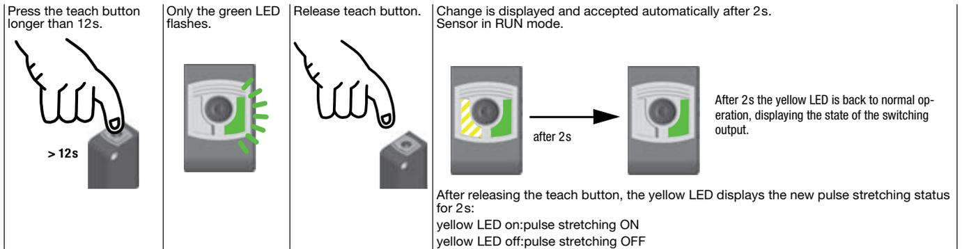
"EasyTune" option - fine tuning of the switching threshold
